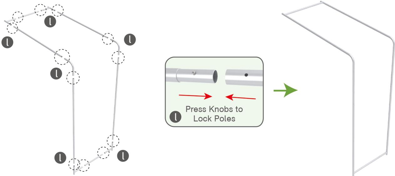
**STEP 03** Connect support poles onto frame.
